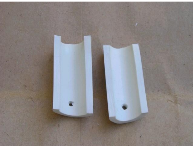
Tubes split, holes drilled, ready to install
