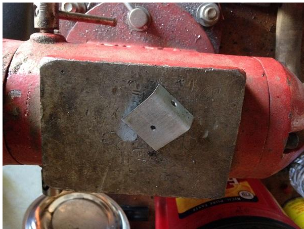
This is the small "L" bracket I made from some scrap metal and drilled 2 holes, one to mount the bracket to the existing tail light housing and the other to anchor the lens.
