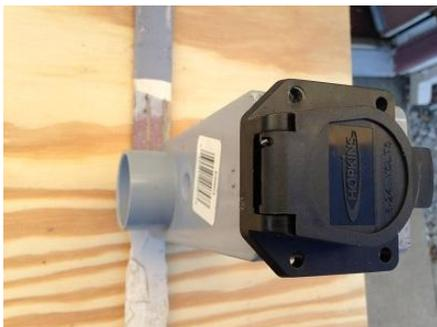
The hole from the cut off flange will have to be reamed out some to allow the trailer connector to slide into the hole.
